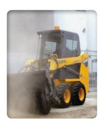
provide up to 38.2 L/min of standard hydraulic flow for powering a wide variety of attachments.
