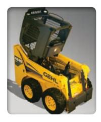
SERVICE IS A SNAP with a swing-open rear door, flip-up engine cover, and tiltable ROPS/FOPS that fully exposes maintenance points at the engine, battery, and filler caps.
