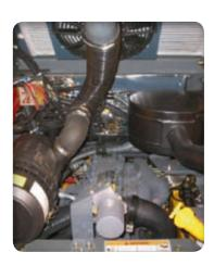
SERVICE IS MADE EASY with a combination of smart engineering and low-maintenance components. The tiltable ROPS/FOPS and large engine cover allow full access to internal components.
