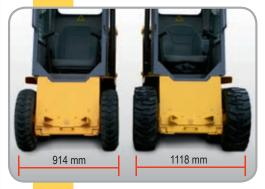
NARROW YOUR OPTIONS – Achieve a super-compact 914 mm width with 5.70 x 12 tire option and 914 mm bucket, or a 1118 mm width with 8.50 x 12 heavy-duty flotation standard tires and 1118 mm bucket.
