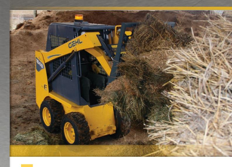
Super-compact and tough, the 1640E skid loader from Gehl can go where other machines can't. A width as narrow as three feet makes maneuvering through narrow doors and alleyways easy, while a strong 386 kg rated operating capacity makes a huge dent in the workload.
