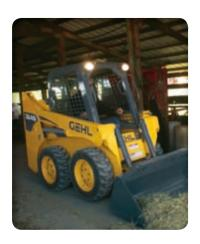
COMPACT MACHINE width as narrow as 1229 mm and overall height just over 1786 mm on the 3840E makes working in tight confines easy.
