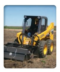
STRONG HYDRAULICS with standard flat-faced couplers provide a high hydraulic flow up to 62 L/min to power a variety of attachments.
