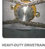
is composed of durable components. Adjustments can be made to the simple "bow-tie" chain system from outside the unit.
