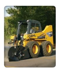
STABLE RIDE is achieved with a longer wheelbase and low center-ofgravity. The HydraGlide<sup>™</sup> ride control option<sup>2</sup> provides smoother operation over uneven surfaces.
