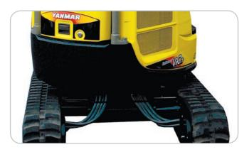
> Layout of the counterweight designed to protect the side panels against any possible shocks.
