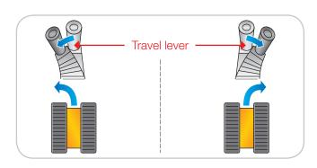
The machine goes according to the orientation of the lever.
